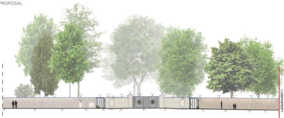
Figure 7.5.10: Existing stone boundary wall treatment onto Sanford Road, as extracted from Cameo&Partners report- denoting the creation of two new pedestrian openings either side of the original gated entrance
