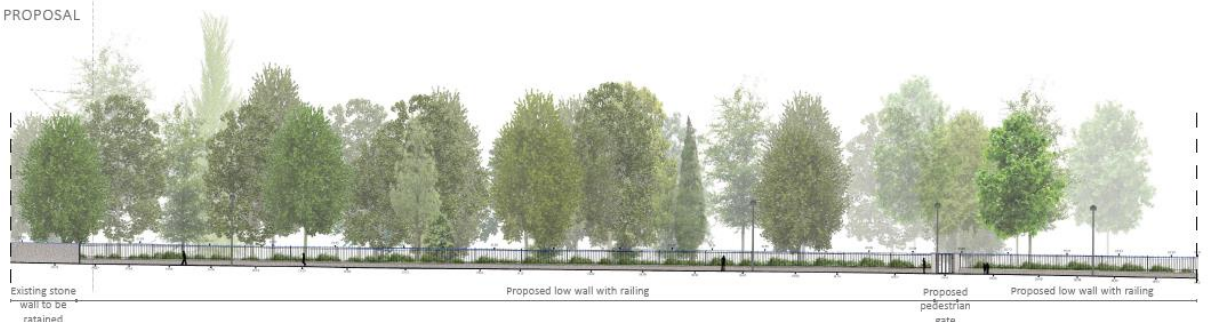
Figure 7.5.8: Existing stone boundary wall treatment onto Milltown Road, extending to junction with Sanford Road (Cameo&Partners)- denoting where original sections of stone boundary wall will be removed and a visually permeable boundary treatment instated
