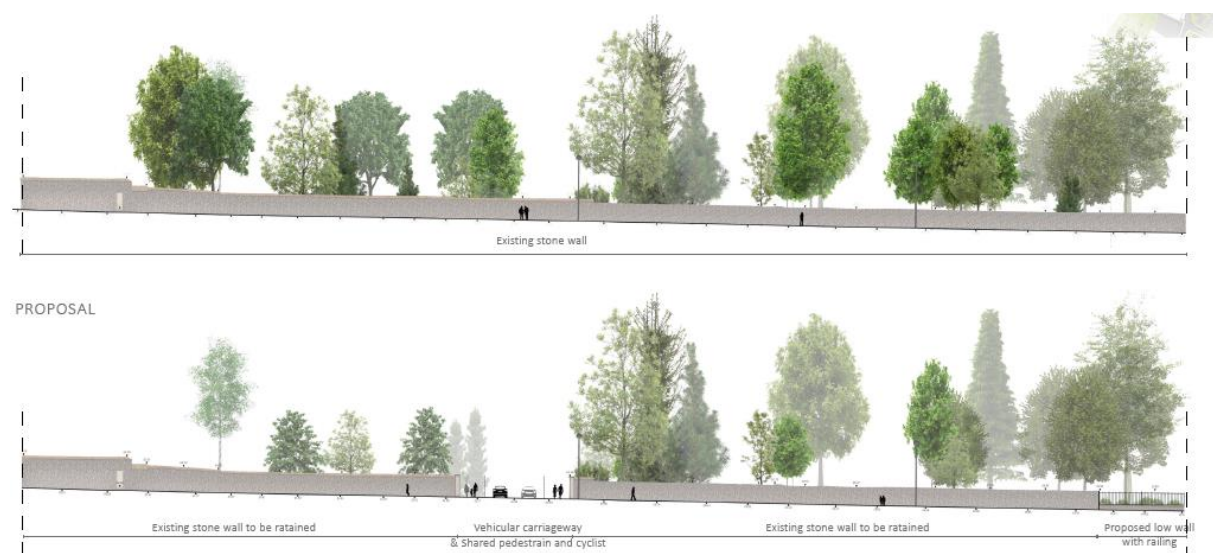
Figure 7.5.7: Existing stone boundary wall treatment onto Milltown Road, (Cameo&Partners)- denoting where a new vehicular opening is proposed
