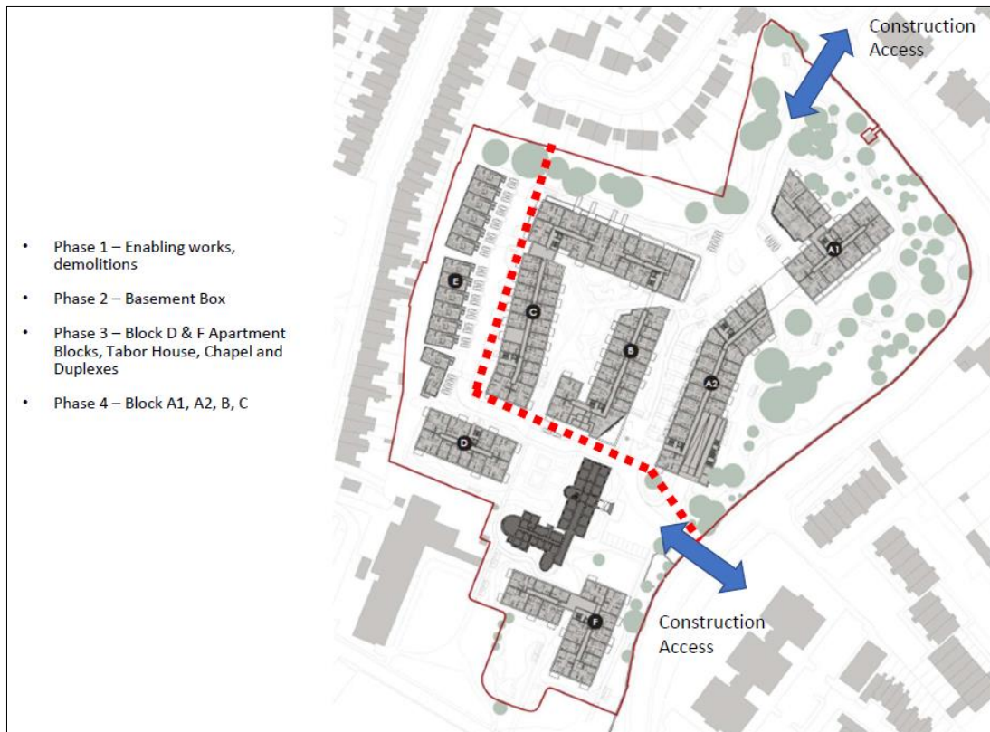
Figure 5.5: Proposed Phasing Plan Layout demonstrating Construction Accesses [Red Dashed Line indicates the Divide Between Phase 3 and 4]
